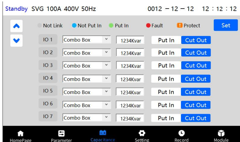
Figure 4.8 Capacitor Switching Control Interface 1
